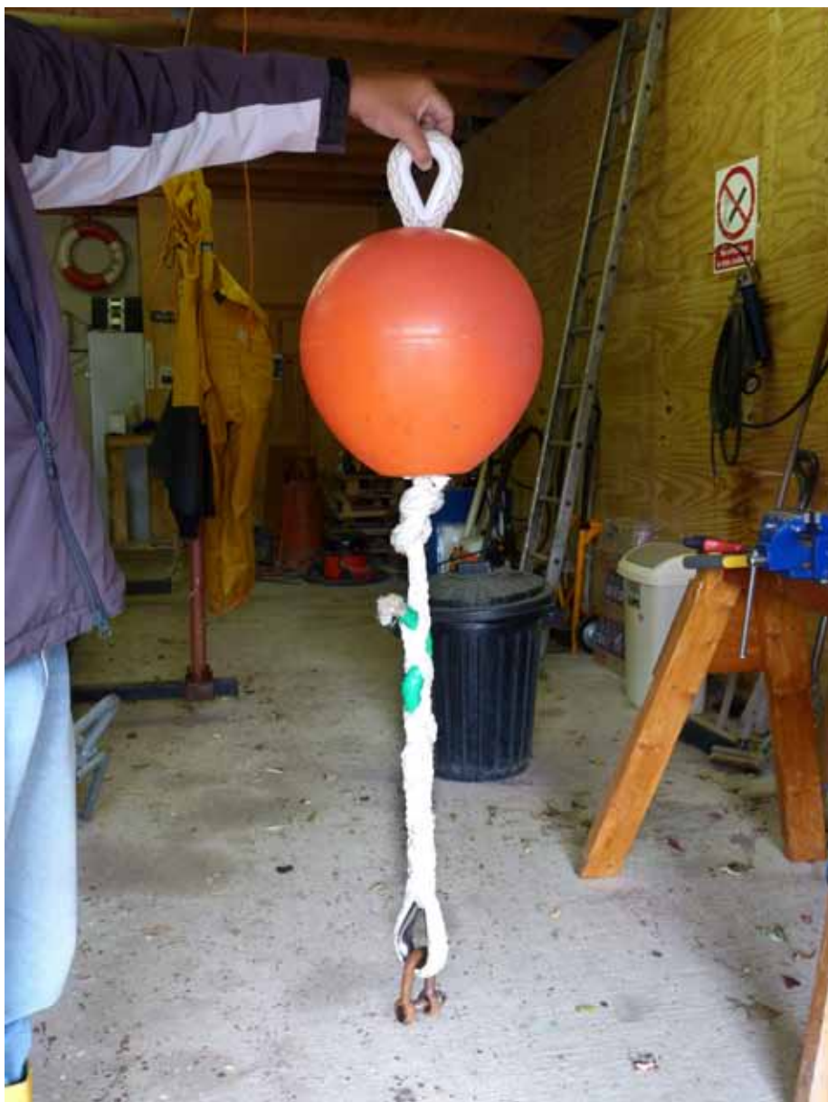
Below: One of the shorter, smaller buoy centres (for a RIB), showing the link to the riser.
