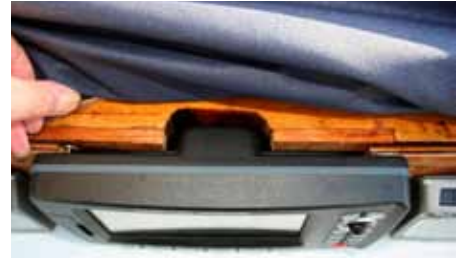
The cutout in the garage houses the GPS antenna and is covered when the sprayhood is erected.
